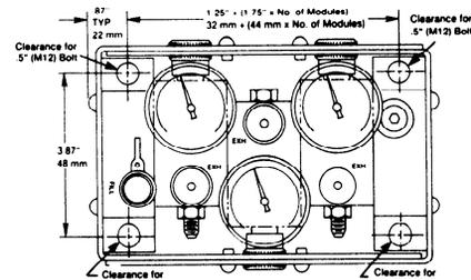
1. The module on the far left must be installed with gauge up as shown.
